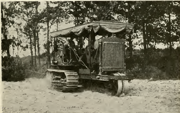
The Holt Caterpillar Tractor. Removes the stump as well as the tree.
